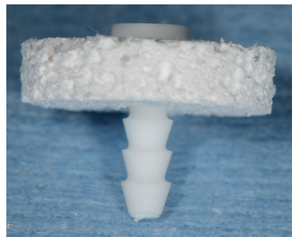
Fig. 1 Graft materials. Fixation pin u-HA/PLLA (1.5 mm in diameter \times 6 mm in length). u-HA/PDLLA composite block (8 mm in diameter \times 2 mm in height)
