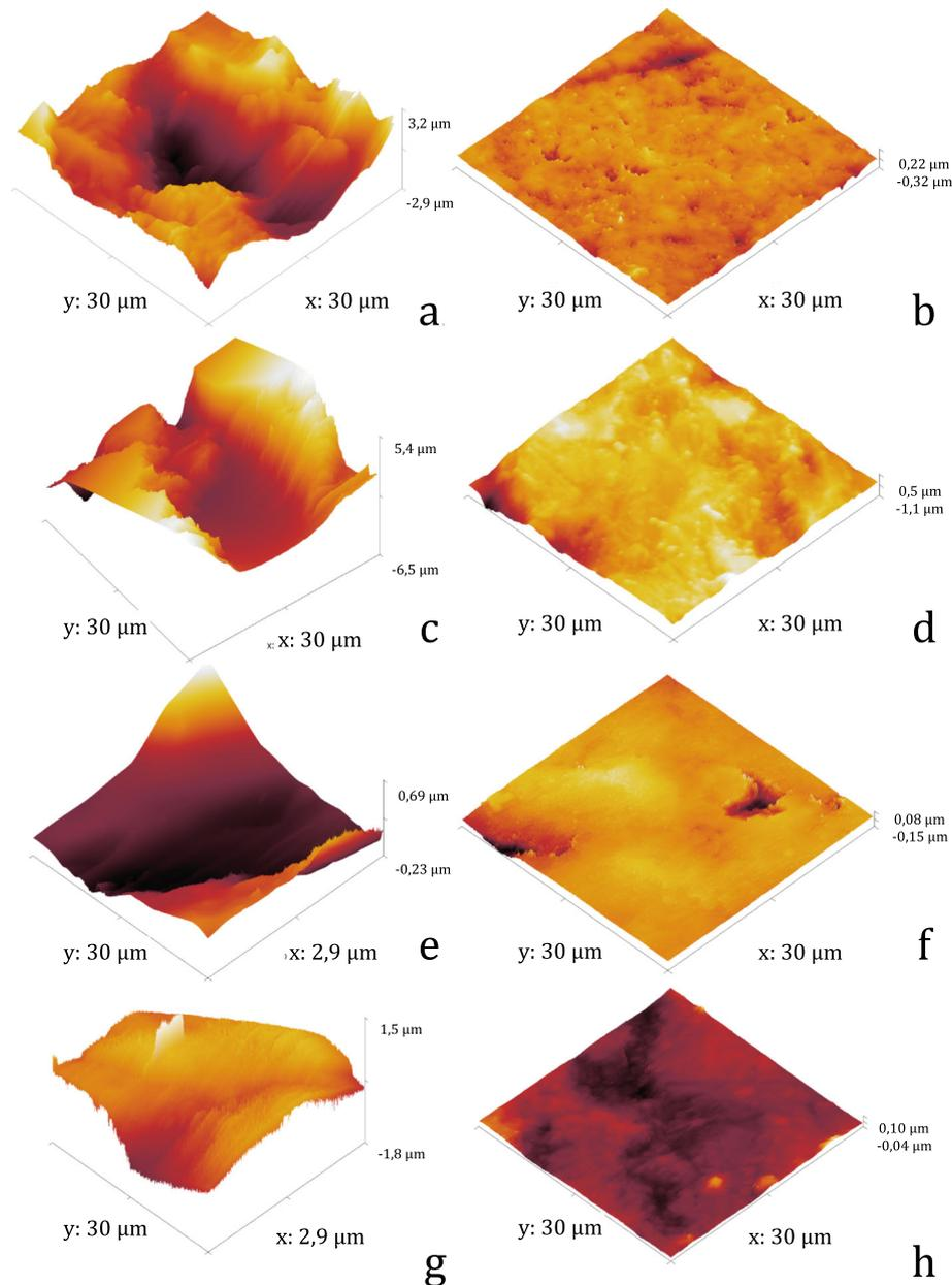
**Fig. 1** AFM images for 30  $\mu\text{m} \times 30 \mu\text{m}$  (a–d) and 3  $\mu\text{m} \times 3 \mu\text{m}$  scan areas (e–h) of rough ceramic (a, e), smooth ceramic (b, f), rough titanium (c, g), and smooth titanium (d, h)
