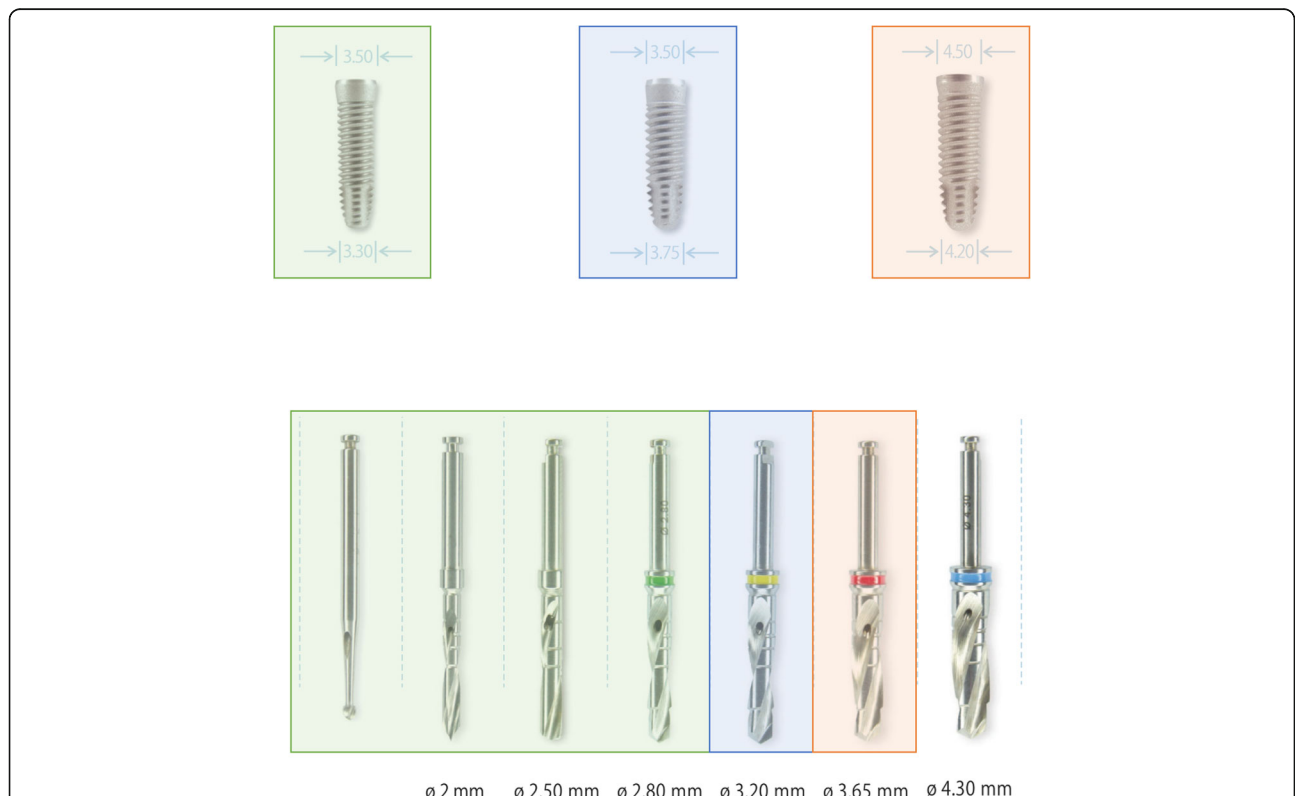
Fig. 1 Standard protocol. This figure shows the implant types and drilling protocol used within this study. Standard protocol was conducted by a final drill of 2.80 mm for 3.3 mm implants, 3.20 mm for 3.75 mm implants, and 3.65 mm for 4.2 mm implants. Permissions for reproducing the figures were received from HI-TEC IMPLANTS LTD. Source: Product Catalogue 12th Edition [40]
