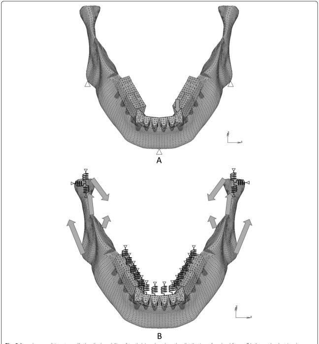
**Fig. 2** Boundary conditions to verify the displaceability of teeth (a) and analyze the distribution of occlusal forces (b). *Arrows*: loads, *triangles*: restricted nodes, *zigzags*: springs
